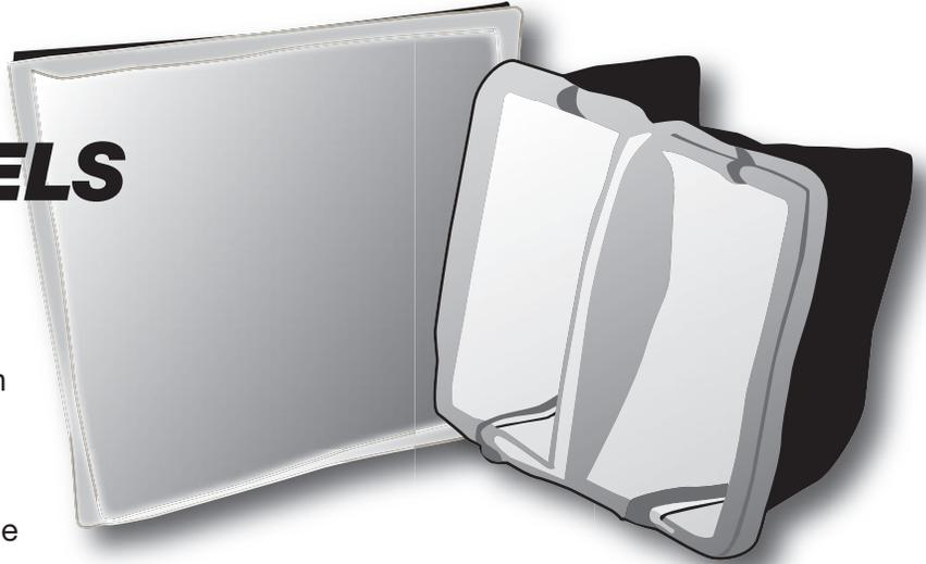
The Two or Three-Ply panels and cubes are constructed of 100% polyester media combined with 3.5 to 5 lbs of activated-carbon impregnated polyester. It is non-toxic, unaffected by moisture and inherently resistant to microbial growth. The polyester and carbon layers are stitched or heat-sealed together with an embedded 9-gauge internal support frame.
