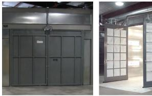
GFS' industrial product doors are constructed with tubular steel frames and structural steel door jambs. Solid doors are covered with a single-skin, 18-gauge steel sheet on the inside face. Filter doors have 18-gauge filter frames for holding filters. Doors include door handles, magnetic closures, foam tape and filters (if applicable). Doors are painted gray or white.
